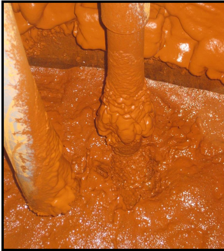
Figure 2-11 Sludge recirculation at the Dawdon mine water treatment plant
